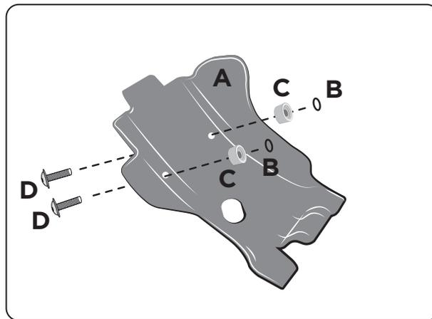
**2. Introduce in the skid plate the screw D, the spacer C and the or B included .**
